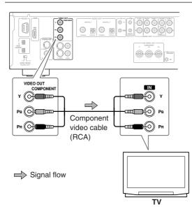
Audio connection not shown here. Make a suitable audio connection to your TV, AV receiver, or amp.
